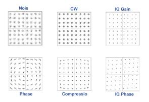
Figure 3. A variety of possible signal pairments. By recognizing the tell-tale signs of different signal impairments, receiver problems can be more easily isolated and debug simplified.
