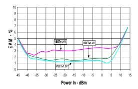
Figure 5. Error Vector Magnitude (EVM) versus input power level for 256-QAM at 1-Msymbol/sec.
