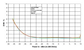
*Figure 7. EVM versus input power for 16, 64, and 256QAM.*
