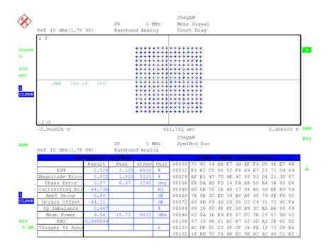
*T*.AUG.2003 11:47:35 Figure 6. IQ constellation of baseband output for 256QAM modulation at 1 Msymbol/sec.
