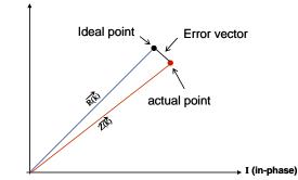
Figure 1. IQ signal space illustrating reference vector, R(k), and measurement vector, Z(k).
