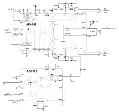
Figure 4. The AD8348 IQ Demodulator in combination with the AD8362 TruPwr<sup>™</sup>Detector can be configured to provide highly accurate automatic level control IF-to-baseband receiver subsystem.
